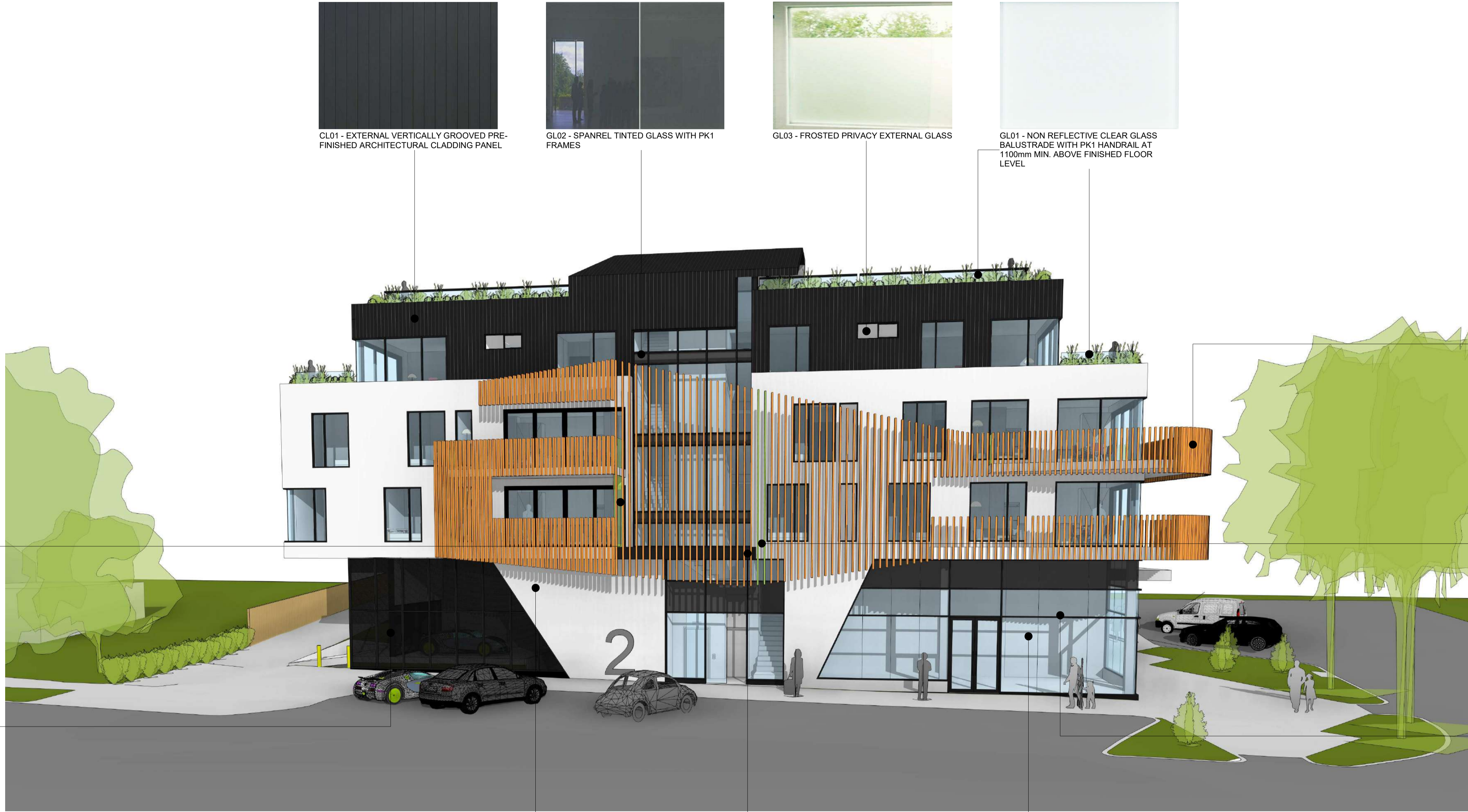
CL02 - PRE-FABRICATED EXTERNAL CLADDING PANEL WITH CONCRETE RENDER FINISH
