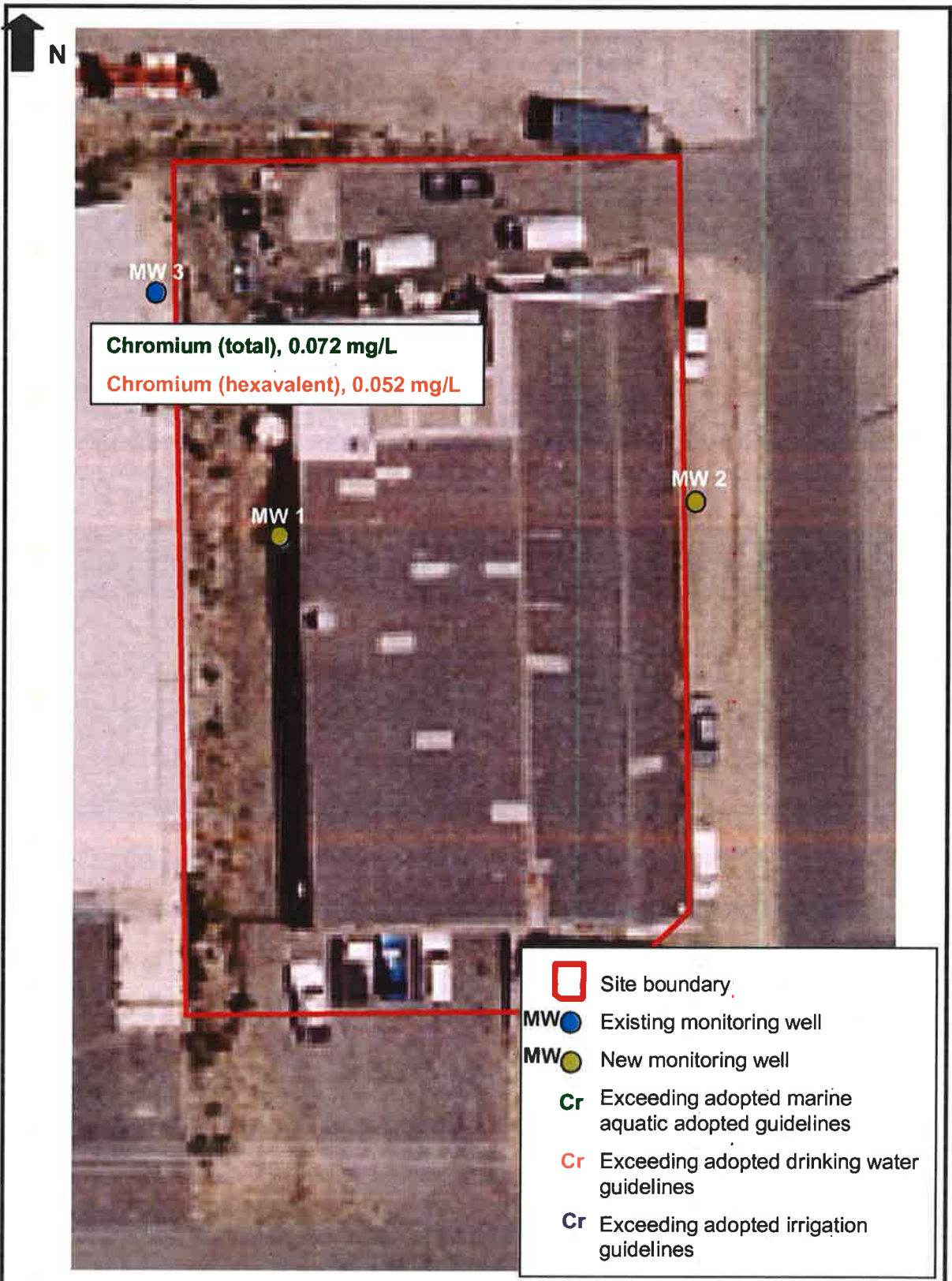
FIGURE 6 : MONITORING WELL LOCATIONS AND EXCEEDENCES
