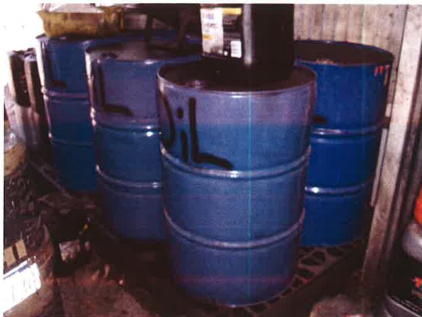
PLATE 5: Chemical storage in unbunded area within workshop
