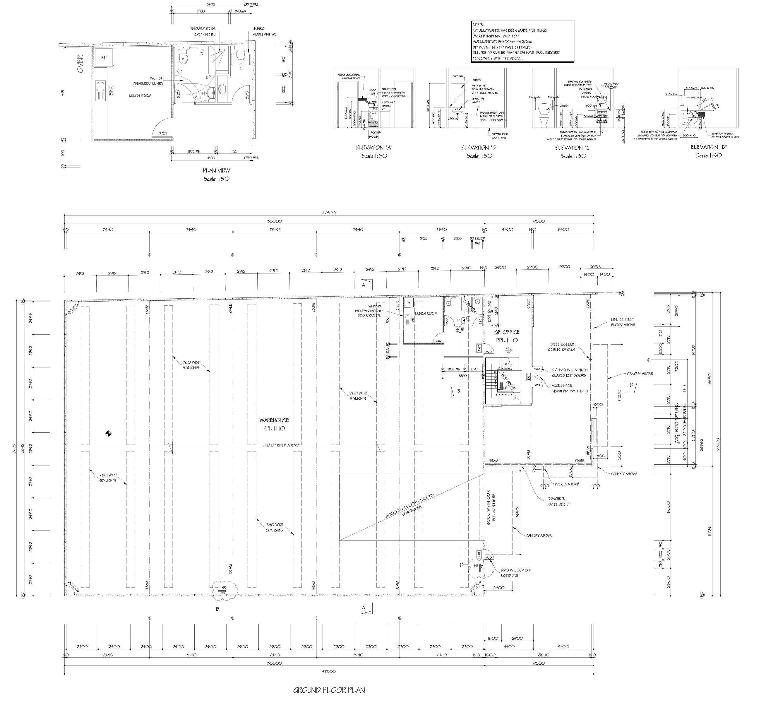
STAIRS TO BE IN ACCORDANCE WITH AS PART D2,13 & D2,14 OF THE NCC 2019 BUILDING CODE OF AUSTRALIA TREADS: 250 MIN, RISERS: 190 MAX.
