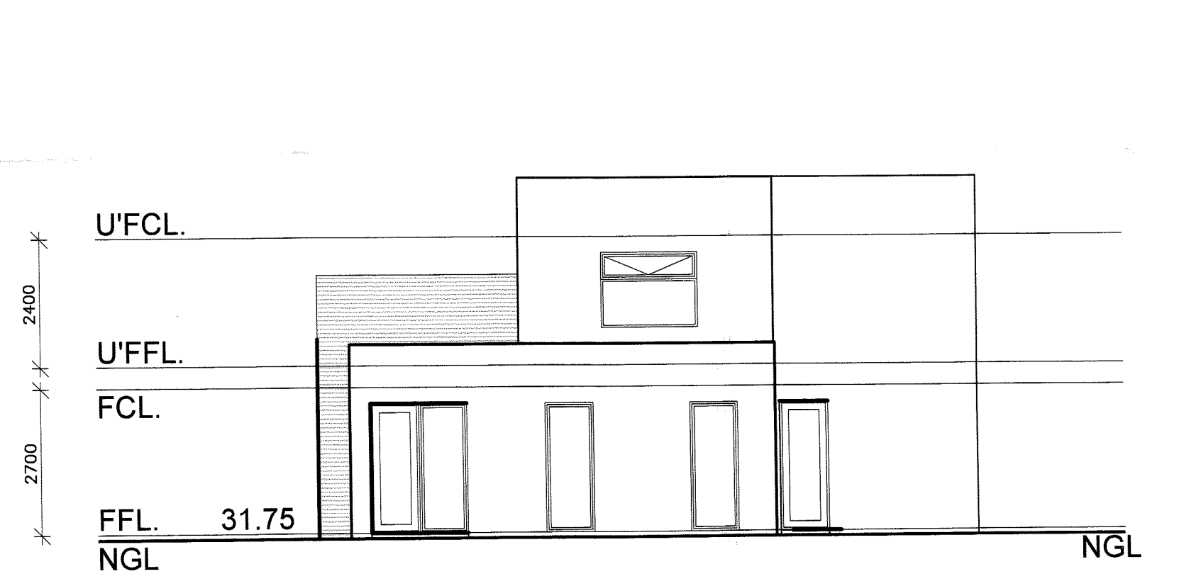
ELEVATION 4 - BREEZEWAY INTERIOR - WEST SCALE 1:100
