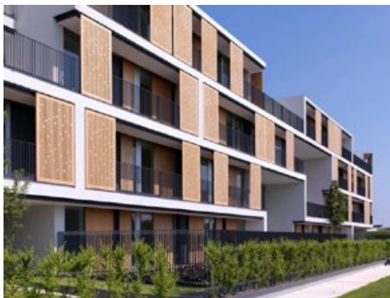
Screening devices can be used to conceal services on balconies as well as provide privacy and shade.
