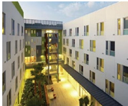
Appropriately sized lightwells can be used to assist solar access, daylighting and ventilation.
