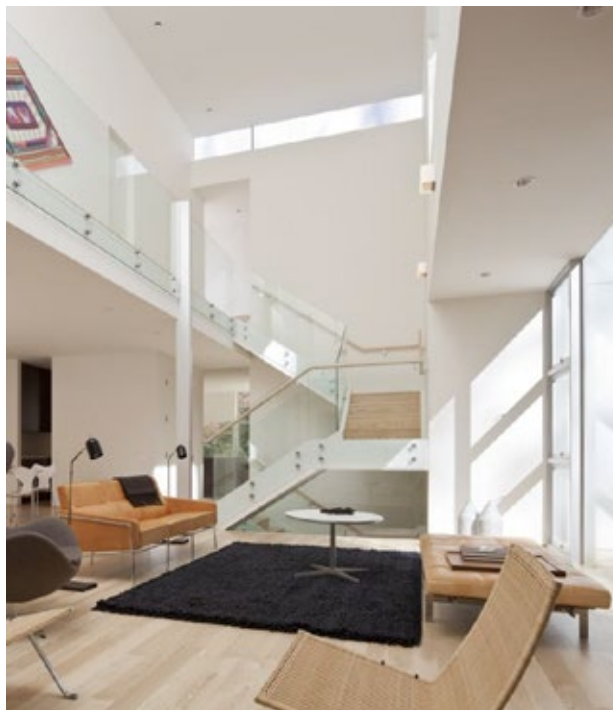
Higher ceilings and high level windows promote daylight access into deeper plans and improve the spatial quality of apartments.
