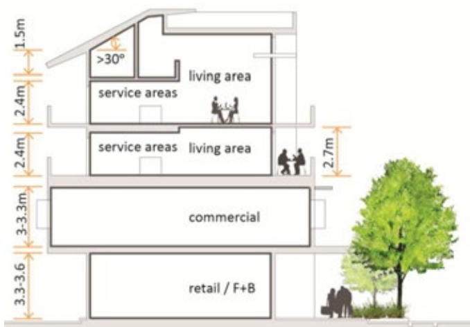
Appropriate ceiling heights for residential and mixed use buildings allowing for 3.3 - 3.6m ceiling for ground floor retail.
