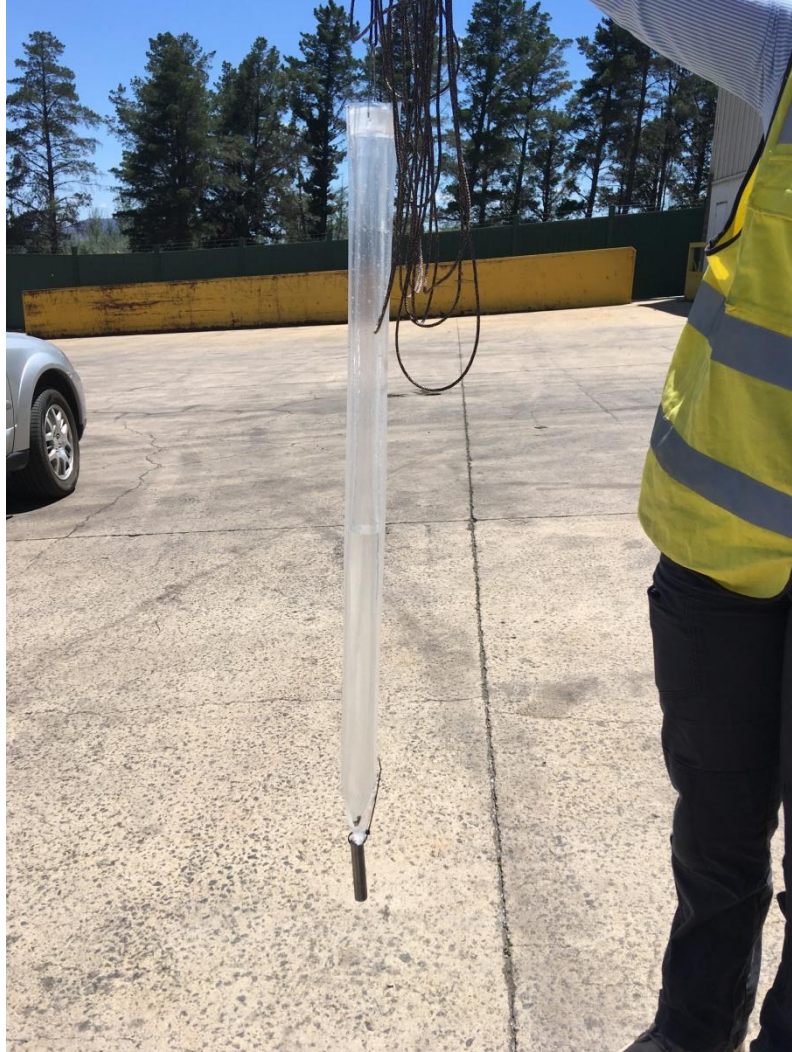
Photograph 4: Groundwater sample collected from monitoring well MW01 (06/12/2018).
